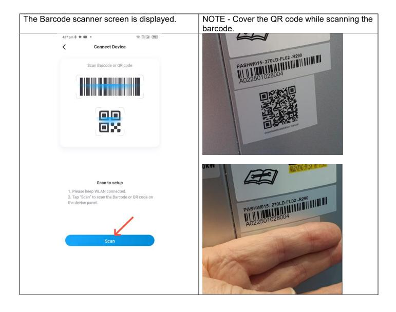
Press the Scan button to scan the barcode on the TANK, please note it is NOT the Wifi module barcode – it is the silver label on the right hand side of the water heater.
