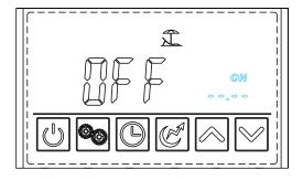
Press and hold the clock button for 2 seconds until the ON, month, and day flashes
