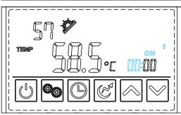
Tap the up or down arrows  $\[ oxedow \]$  to adjust the **ON 1** hour
