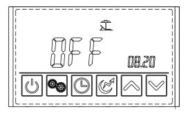
Press and hold the power button for 2 seconds then release to switch the unit off
