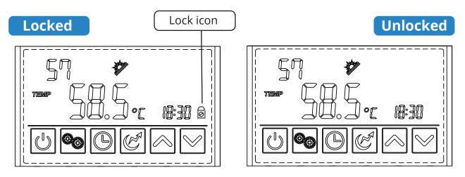
To unlock the screen simply press and hold the power button for 6 seconds.
