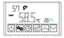
Tap the clock button (5) to complete the timer setting
