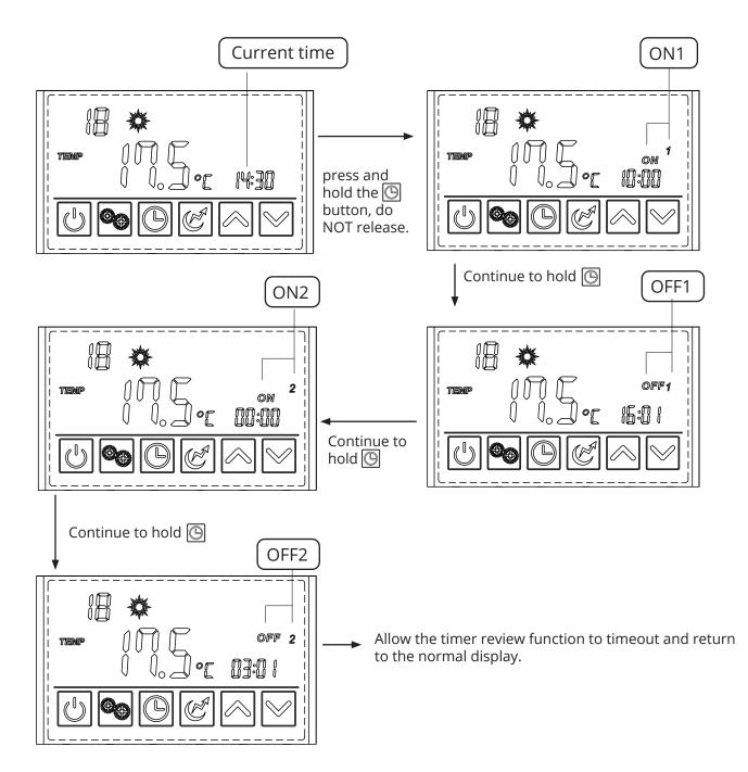
NOTE: Do not set the second timer to 00:00 ON and 00:00 OFF as the unit will commence heating at midnight every second night. To leave the second time off simply allow the timer setting to time-out after setting the first timer end time.
